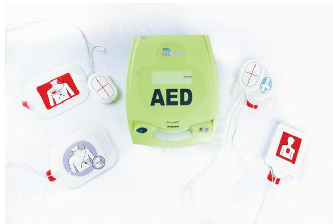
Figure 4-12 | Some AED models come with pediatric AED pads that are smaller and deliver lower levels of energy, whereas others have a pediatric setting or key instead of specific pediatric pads. As always, follow the manufacturer's recommendations and your facility's protocols.
