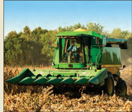
**Fig. 22-27:** Combine parts such as the auger, heads, reels and snapping rollers can cause serious injuries. *Courtesy of Michelle Lala Clark.*
