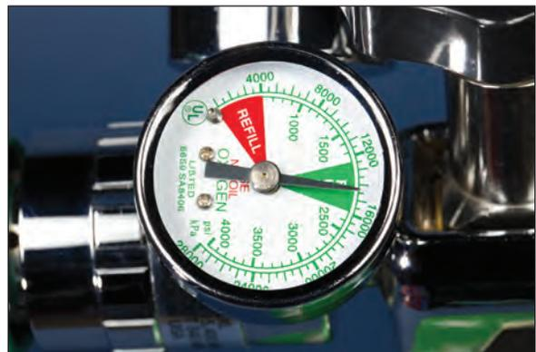
**Fig. 12-3:** A pressure regulator is attached to an oxygen cylinder to reduce the pressure of oxygen to a safe level.
