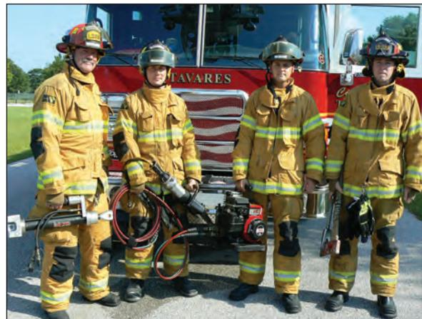
**Fig. 28-7:** Extrication tools, used to access patients, include hand tools, pneumatic tools, hydraulic tools, cutters and rams. *Courtesy of Ted Crites.*
