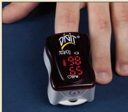
**Fig. 8-19:** A pulse oximeter measures the oxygen saturation level in a patient's blood.
